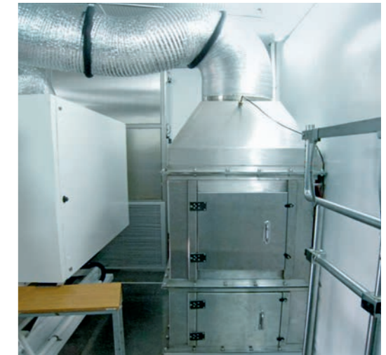
The R&D facility also has psychrometric test facilities to conduct performance tests in line with international testing standards.
